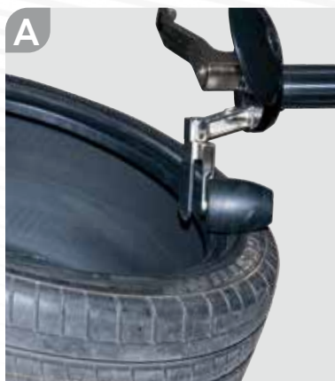
A-B. The upper BEAD BREAKER DISC and built-in plastic roller push the tyre into the rim.
