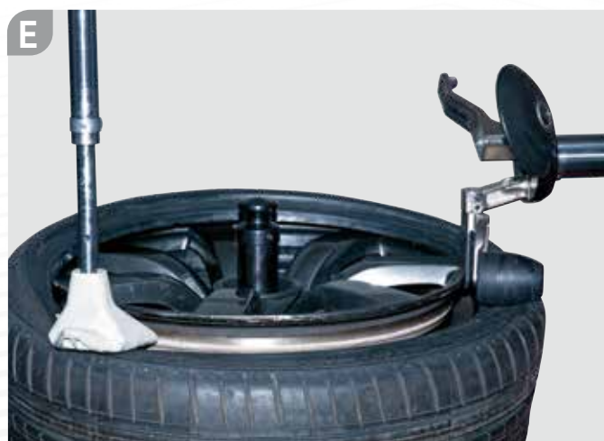
E-F. By positioning the REVOLVER mounting tool head between the rim and the tyre, the REVOLVER PLASTIC ROLLER will automatically help the tyre to stay in the channel.
