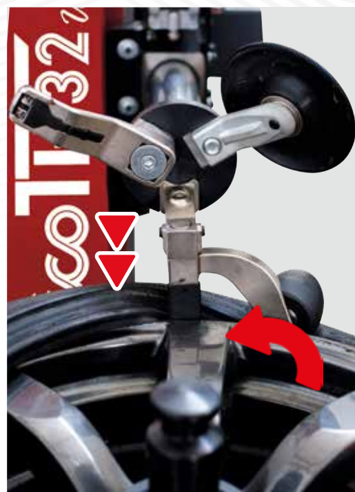
Complete MOUNTING operation facilitated by tool and built-in presser always in the same position.
