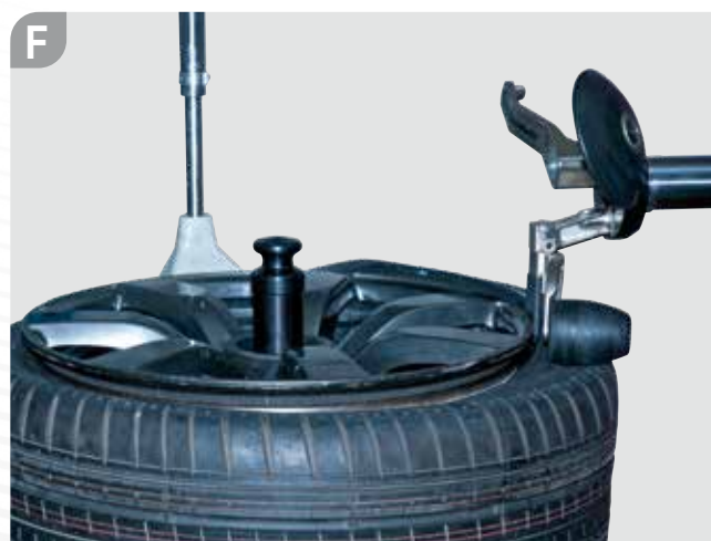
E-F. By positioning the REVOLVER mounting tool head between the rim and the tyre, the REVOLVER PLASTIC ROLLER will automatically help the tyre to stay in the channel.
